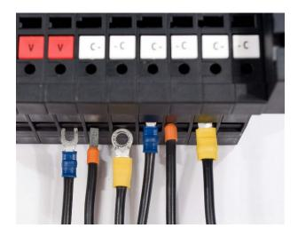
Recommended wire gauge is from 1.5 mm<sup>2</sup> (AWG 16) to 4 mm<sup>2</sup> (AWG 12).
