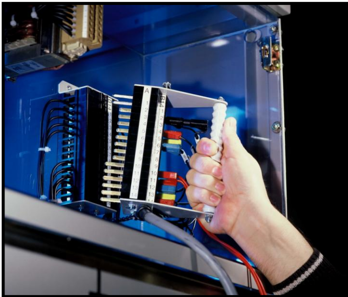
Image 7: SecuControl interface test system
